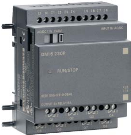
LOGO! DM16 230R MOD.AMPLIACION, AL/E/S: 230V/230V/RELE, 8 ED/8 SD, 4 MODULOS
