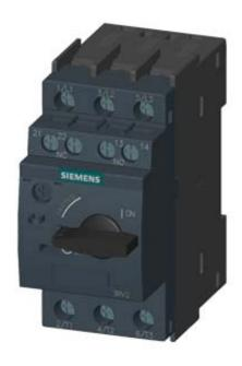
CIRCUIT-BREAKER SZ S0, FOR MOTOR PROTECTION, CLASS 10, A-RELEASE 11...16A, N-RELEASE 208A, SCREW CONNECTION, STANDARD SW. CAPACITY, W. TRANSVERSE AUX. SWITCH 1NO+1NC
